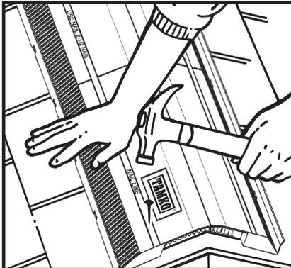
**3.** When reaching the other end, the last vent section may need to be cut to length. End plugs are provided every 12" on underside of the product. Measure amount needed to install to within 1" of gable end. Cut that length in from end of vent section and flip around so that end plug is at gable end. Allow male tab from previous piece to slide under last piece and nail in place.
