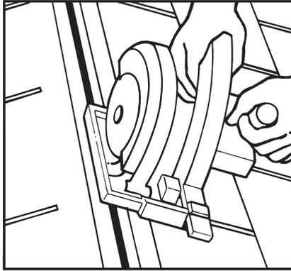
**2.** Place first piece of vent with female end 1" in from gable end and use centering line for proper alignment along peak. Fasten using at least two nails at each end and in the middle of section in nail line area (2-1/2" minimum nail length). More may be required on steeper slopes to seat properly. Continue installing additional pieces along ridge sliding female end over male end, aligning using centering line.
