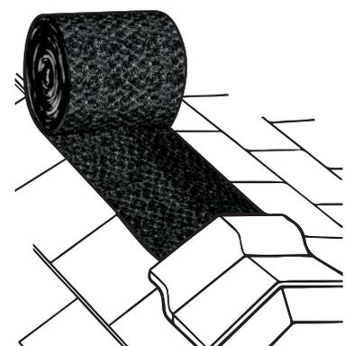
3. Center ridge cap shingles over vent and install with minimum 1 3/4" nails. Assure nails penetrate into sheathing 3/4" or completely through sheathing. Cap shingles can be laid down over end of vent onto ridge out to gable ends.
