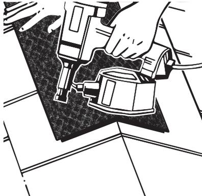
2. No end cap is necessary if ridge cap shingles are lapped over end of product and down onto ridge. In this case, run vent to 12" from gable ends. Center vent over slot at one end with flat side facing up. Fasten with two nails; minimum nail size of 1 3/4". If using nail gun, recommended compressor pressure is between 90 and 100 psi. Roll out length of ridge, pull out slack, and fasten with two nails at opposite ends.
