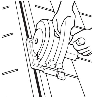
1. Snap chalk line and cut a slot 2" wide total along ridge (or 1" on each side of ridge beam). Allow for a closed area of sheathing 18" at both ends of ridge.
