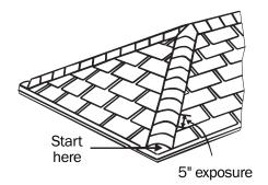
Secure each shingle as illustrated in Figure 2 with one fastener on each side, 5-1/2" back from the exposed end and 1" up the from the edge. The length of the fastener should be long enough to penetrate through the roofing material and 3/4" into the wood decking or completely through the decking.
