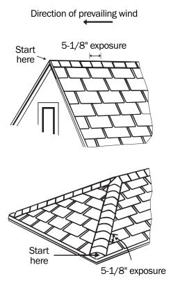
Secure each shingle as illustrated in Figure 2 with one fastener on each side, 5-5/8" back from the exposed end and 1" up the from the edge. DO NOT NAIL BELOW THIS LINE 1" UP FROM THE EDGE. The length of the fastener should be long enough to penetrate through the roofing material and 3/4" into the wood decking or completely through the decking.
