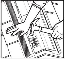
sliding female end over male end, aligning using centering line. NOTE: In cold weather, allow 1/8" gap between vent sections for expansion.
