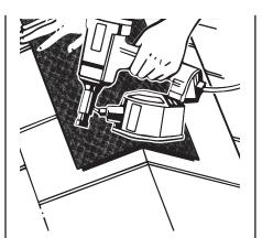
2. No end cap is necessary if ridge cap shingles are lapped over end of product and down onto ridge. In this case, run vent to 12" from gable ends. Center vent over slot at one end with flat side facing up. Fasten with two nails; minimum nail size of 1 3/4". If using nail gun, recommended compressor pressure is between 90 and 100 psi. Roll out length of ridge, pull out slack, and fasten with two nails at opposite ends.
