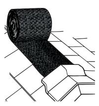
3. Center ridge cap shingles over vent and install with minimum 1 3/4" nails. Assure nails penetrate into sheathing 3/4" or completely through sheathing. Cap shingles can be laid down over end of vent onto ridge out to gable ends.
