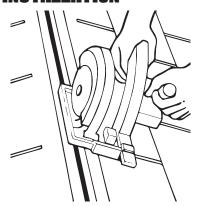
Snap chalk line and cut a slot 2" wide total along ridge (or 1" on each side of ridge beam). Allow for a closed area of sheathing 18" at both ends of ridge.
