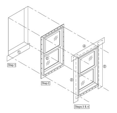
Figure 1: Window installation detail for windows with integral flanges and flashing installed prior to WRB
