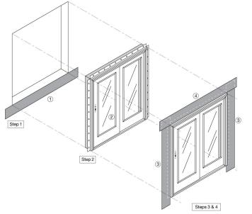
Figure 3: Door installation detail for doors with integral flanges and flashing installed prior to WRB
