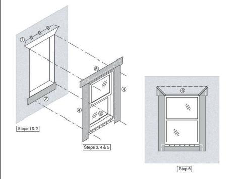
Figure 2: Window installation detail for windows with integral flanges and flashing installed after WRB
